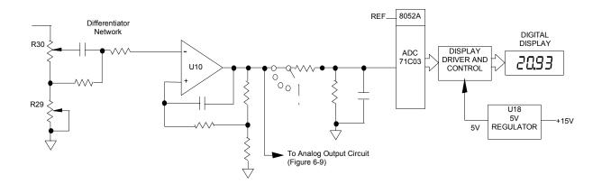
Figure 5-9. Buffer, Anticipation, and Digital Output Circuit
